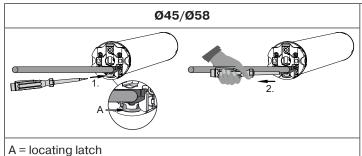
Insert a suitable flathead screwdriver right into the recess of the locating latch, so that the latch releases the locating lug from the plug.
